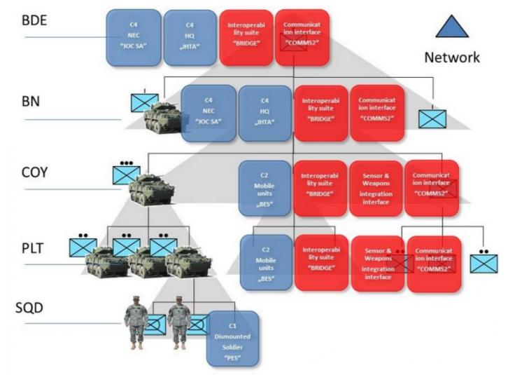
Basic requirement for any C4I system is to support a full digital line of command from the HQ, down to the dismounted soldier. MIL C4I Battle system, delivers that functionality along, with specially tailored user interface, and set of features for every level.
