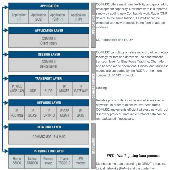
transmitted data. COP sharing, Messaging, Blue Force Tracking, Targeting, Chat etc. is distributed over the COMMS2 layer by the WFD protocol.
