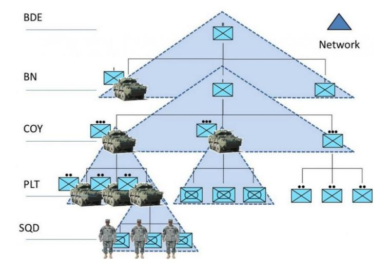
WFD will take advantage of radio network physical specifics, and will broadcast the data to all the nodes in the same network. Unit commanders, that are present in upper and lower network at the same time, act as gateways which aggregate the information and resend only the relevant data in order to keep the traffic at minimum. Although "lateral communication" between neighboring units is technically possible via COMMS2 routing or rebroadcast functionality it is generally avoided.
