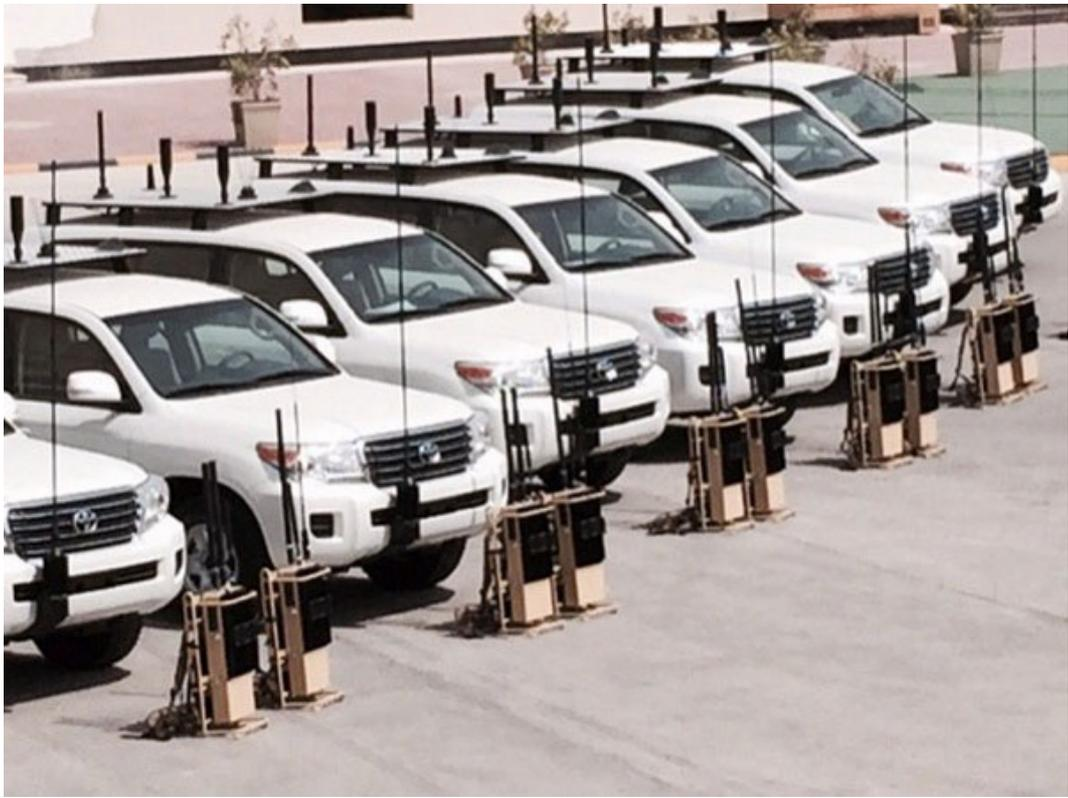
The system is equipped with 3 omni-directional antennas. VHF module and UHF module have its own antennas. RF outputs of upper bands (3 and 4) are combined into one high gain collinear dipole antenna. The lowest feed point of this antenna is elevated about 250 mm from the base of the antenna, allowing the signal to be radiated over the user's head. This reduces absorbed power and increases field strength at the target (i.e. no need for additional antenna elevation).
