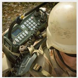
The waveform is based on the Standard NATO Agreement (STANAG 4538) and is available as an option for the Codan's 2110M series HF man pack radio. The (3G) automatic link establishment (ALE) supports enhanced data throughput and linking performance over noisy HF Skywave channels. Integratio of the ALE linking protocol and the data transport mechanism provides effective increased data throughput and shorter linking times in difficult HF conditions.
