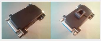
The AT Voice USB-Logger is a simple device designed to provide time stamped recording and metatag logging of voice and data communication. The AT USB-Logger includes a simple software program installed on a PC that connects through the AT Voice USB-Logger to your communication transceiver eg Codan Envoy or NGT.
