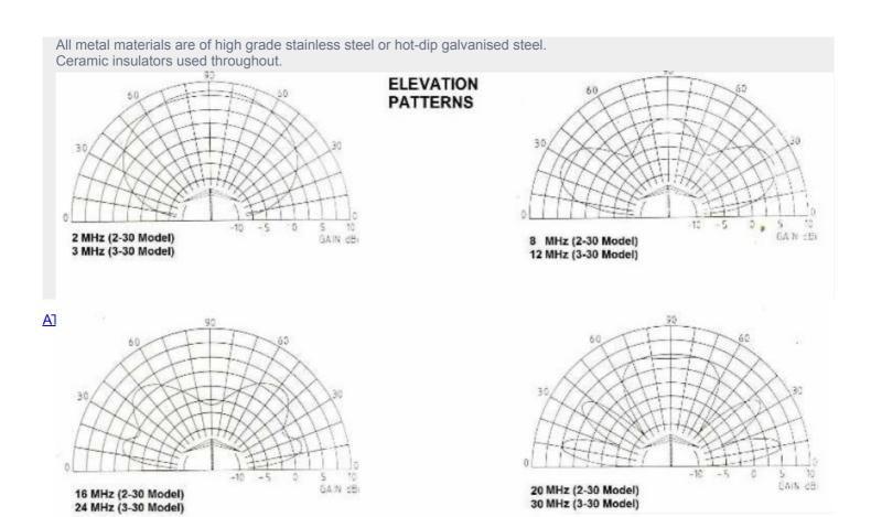
AT HF Biconical Dipole Antenna
