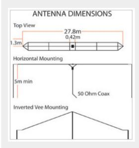
High efficiency broadband multi-wire base antenna. Sturdy stainless steel and fiberglass construction, can be mounted horizontally or as inverted V. Supplied with 30m of co-axial cable and instructions.
