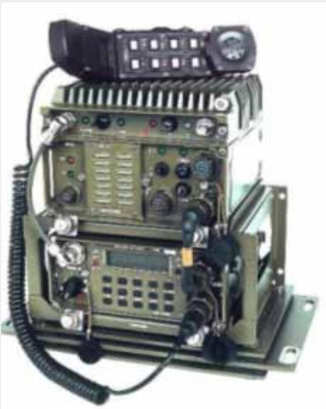
This mobile package with maximal output power of 25 W can be installed in all wheeled and tracked vehicles. The AT RF13 transceiver and ATZM13.1 amplifier are located on top of each other in a springcushion frame. If the mobile set is designed for installation in wheel vehicles without artillery or mortar weaponry, c for fixed posts, you may use the lighter, non-cushioned frame 7007.100.01 instead of springcushion frame 7007.100.10. The set can be controlled from one location.
