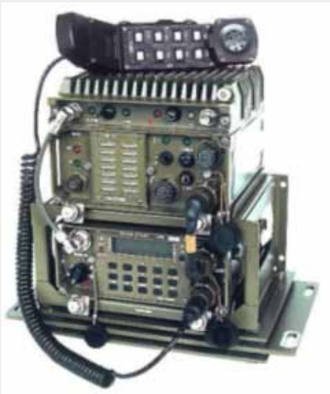
This mobile package with maximal output power of 50 W can be installed in all wheeled and tracked vehicles. The AT RF13 transceiver and AT ZV13.1 amplifier are located on top of each other in a spring cushion frame. If the mobile package is designed for installation in wheel vehicles without artillery or mortar weaponry, or for fixed posts, you may use the lighter, non-cushioned frame 7007.100.01 instead of spring cushion frame 7007.100.10. The package can be controlled from one location.
