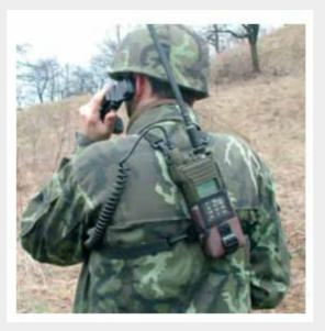
AT RF20 ECCM handheld multiband transceiver with improved resistance to electronic warfare is designated for use at the lowest tactical command levels for all kinds of military units. Depending on the type of selected frequency band, the transceiver is able to communicate in HF band with frequency modulation, with VHF AT RF13 transceivers AT RF2050 mobile transceivers and with airborne transceivers in Aircraft band I.
